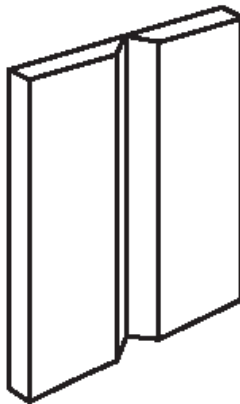
(C) VERTICAL WELDING TEST POSITION 3G
